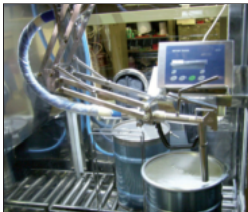
Isolatore con dispositivo di pesata e carico sostanze liquide in fusti Glove box with weighing device for charging of liquid into drums
