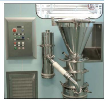
For the use in classified area (in presence of dangerous gas/dust mixtures) it is available an "ATEX" version suitable for installation zone 1-21 or 2-22 as per the directive 94/9/EC.
