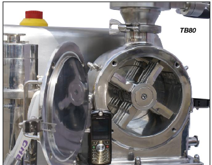
To grant a radical cleaning all parts in contact with the product are realized in stainless steel AISI 316L and mirror polished.
