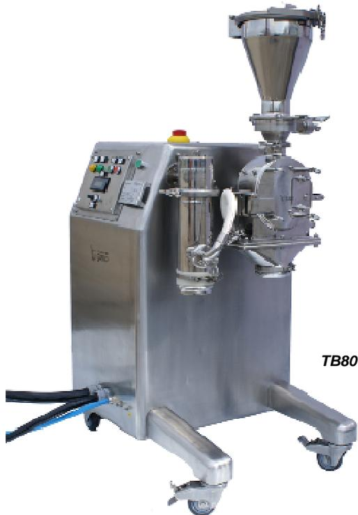
The hammer mill "TURBINE" is available in three different models, suitable for treatment of product batches from 0,1 kg/h (laboratory version) up to 2000 kg/h, reaching finenesses lower than 100 micron.
